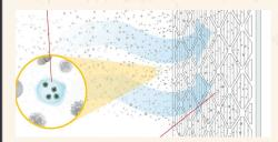
Air filters with a rating of MERV 13or higher capture airborne particles between 0.3 and 1.0 microns.
