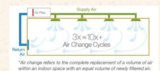
Install air filters with a minimum MERV 13 rating, as per ASHRAE 52.2-2017, in each ventilation system supplying outdoor air to occupied spaces. Other options to achieve this credit may include filters that can withstand increased ventilation/airflow rates and the removal of contaminants from exhaust air though gas-phase filters and/or containment systems.
